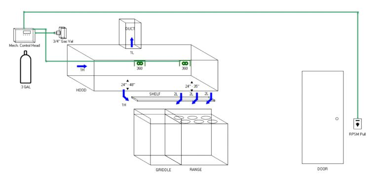
Existing fire system is being replaced with a new Protex L3000 system with a 10 flow point capacity. This application uses 9 flows. System uses 3/8" black steel piping, fusible metal links, automatic gas valve, remote manual release by exit door, switches for supply air shutdown. Hood - 8'L x 4'W
