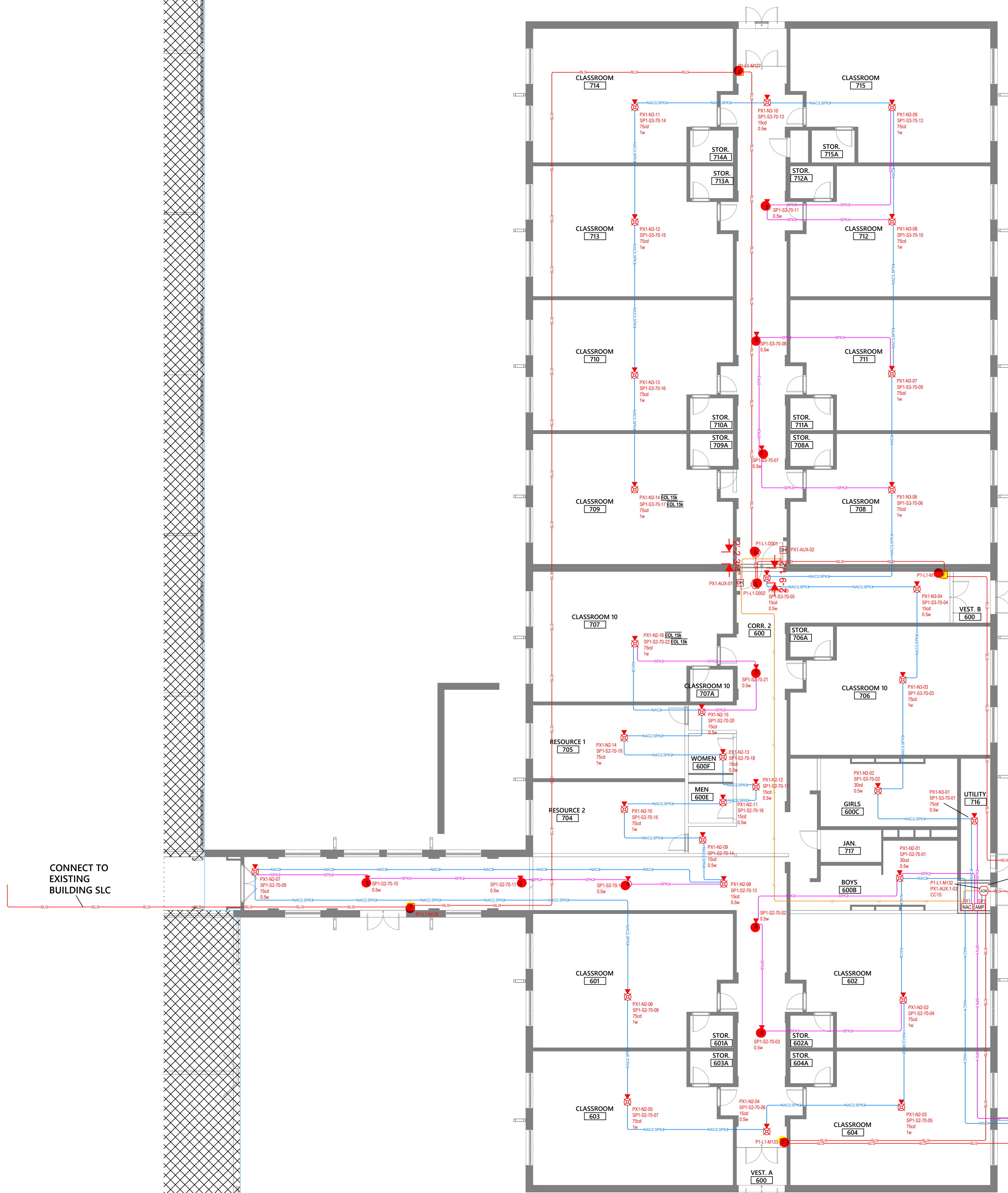
1 FIRST FLOOR FIRE ALARM SCALE: 3/32" = 1'0"
