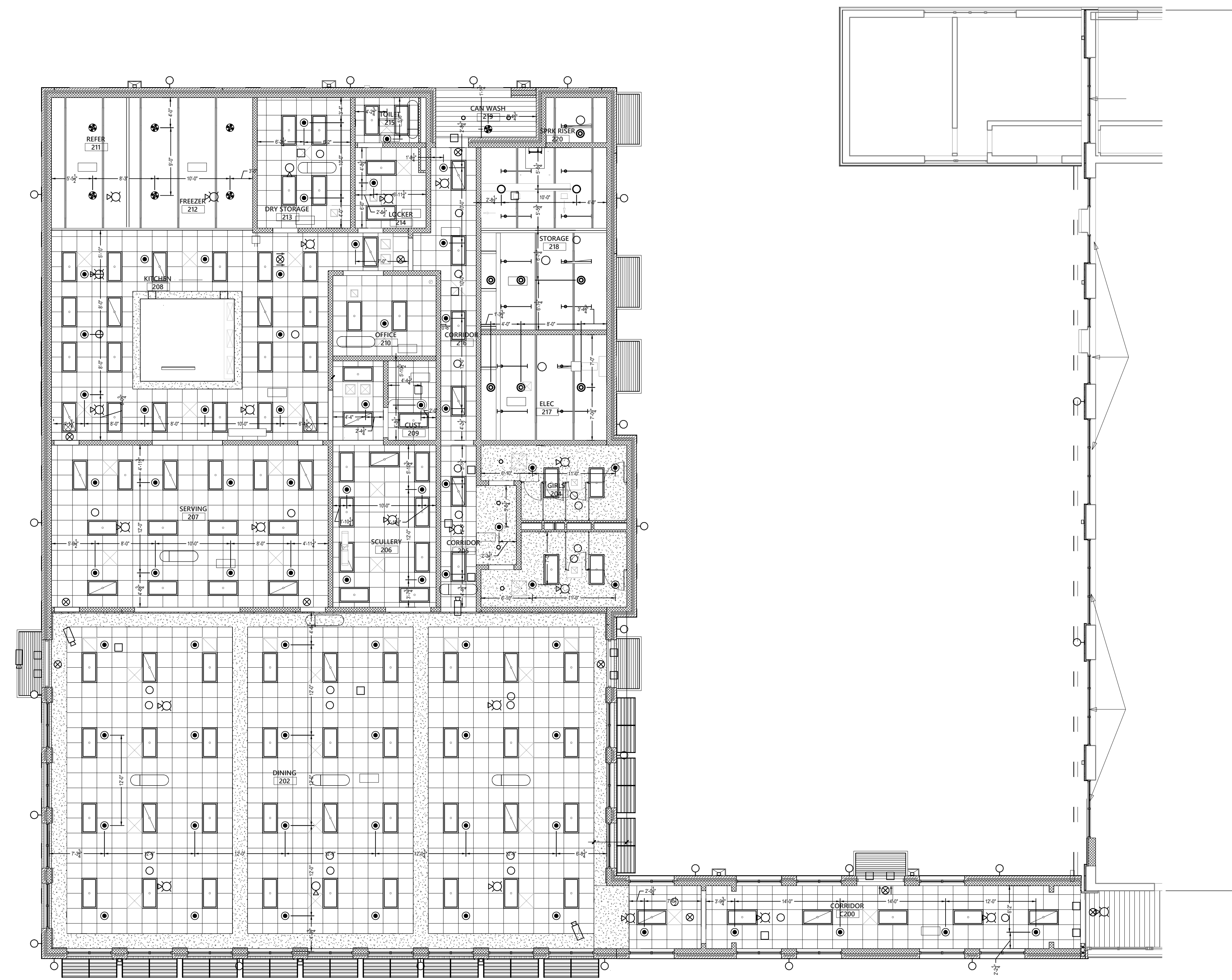
SPRINKLER SYSTEM - HEAD LAYOUT SCALE: 1/8" = 1'-0"
