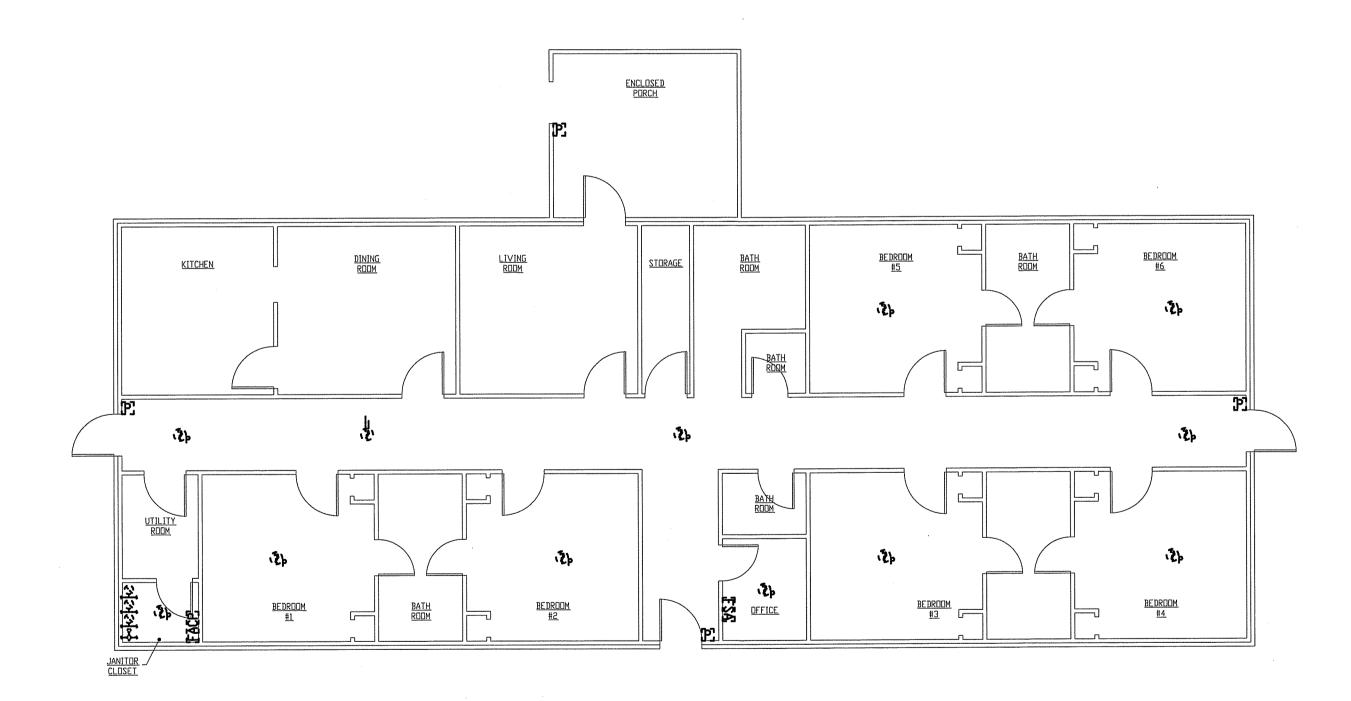
INSTALLATION OF HEAT DETECTORS IN ATTIC OF BUILDING AS REQUIRED BY AHJ. FIRE ALARM SYSTEM IN LIVING AREA OF BUILDING HAS BEEN INSPECTED AND PASSED.
