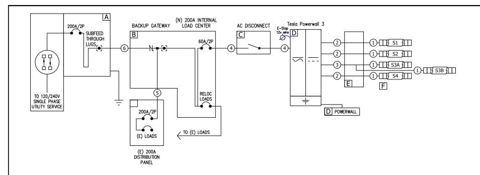
MAIN SERVICE PANEL IS COMPLIANT WITH NEC 705.12(B)(2)(3)(c)
