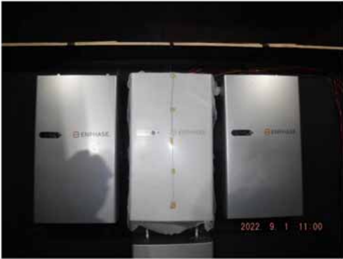
Figure 2: Initiating unit in the middle covered with cheesecloth together with the target units
