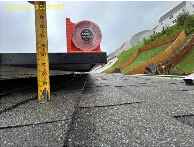
Roof Photos / Array 2 / Tilt - measured on array
