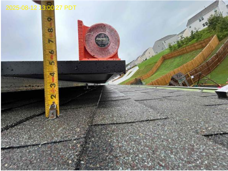
Roof Photos / Array 1 / Tilt - measured on array
