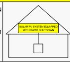
NEC 690.56 (C)(1)(a) PLACE WITHIN 3FT OF SERVICE DISCONNECTING MEANS TO WHICH THE PV SYSTEMS ARE CONNECTED AND SHALL INDICATE THE LOCATIONS OF RAPID SHUTDOWN SWITCHES
