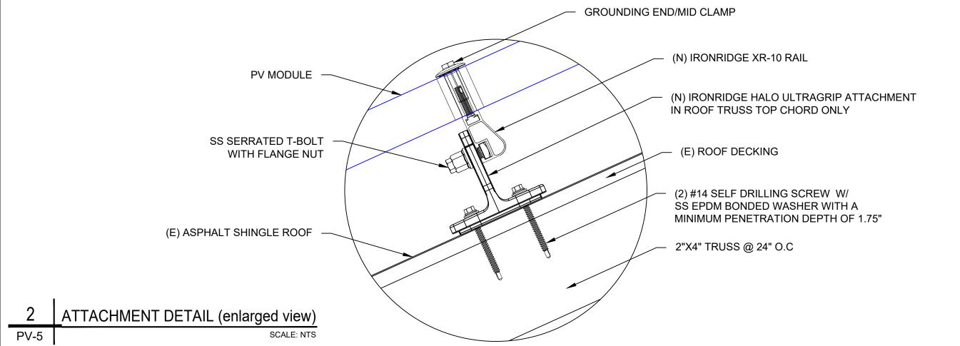
DC SYSTEM SIZE: 5.265 kW DC AC SYSTEM SIZE: 5.700 kW AC (13) JA SOLAR: JAM54S31-405/MR 405W MONO MODULES WITH (13) SOLAREDGE: S440 POWER OPTIMIZERS LOCATED UNDER EACH PANEL (240V) AND (01) SOLAREDGE: SE5700H-US (240V/5700W) INVERTER (01) STRING OF 13 MODULES ARE CONNECTED IN SERIES **INTERCONNECTION NOTES:**
