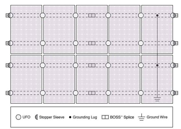
Approved Enphase microinverters can provide equipment grounding of IronRidge systems, eliminating the need for grounding lugs and field installed equipment ground conductors (EGC). A minimum of two microinverters mounted to the same rail and connected to the same Engage cable is required. Refer to installation manuals for additional details.
