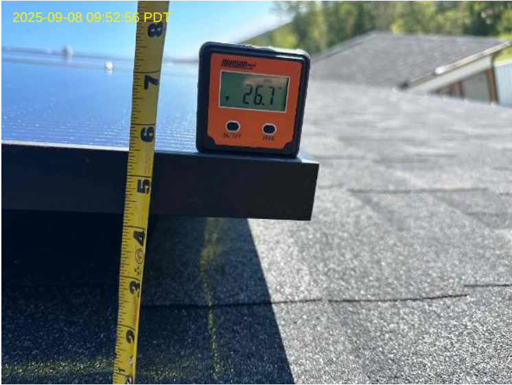
Roof Photos / Array 1 / Tilt - measured on array
