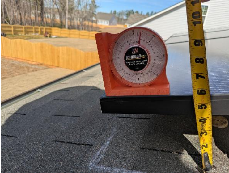
Roof Photos / Array 2 / Tilt - measured on array
