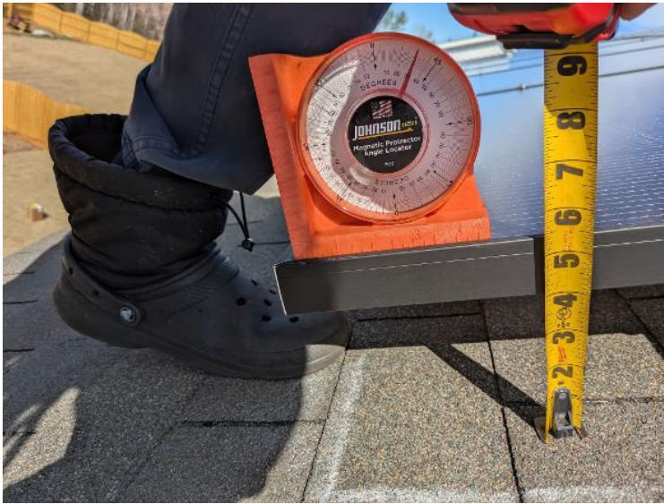
Roof Photos / Array 1 / Tilt - measured on array
