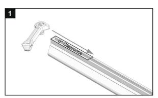
Slide CAMO into rail channel far enough to clear the module frame. CAMO requires 6" of clearance from end of rail.
