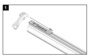
Slide CAMO into rail channel far enough to clear the module frame. CAMO requires 6" of clearance from end of rail.
