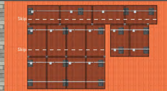
Example of Tile Roof Array
