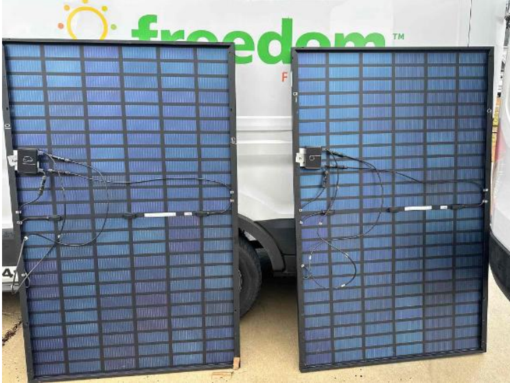
Rooftop Installation / 2 Optimizer's/ Micro Inverter's/ Tesla MCI's Installed
