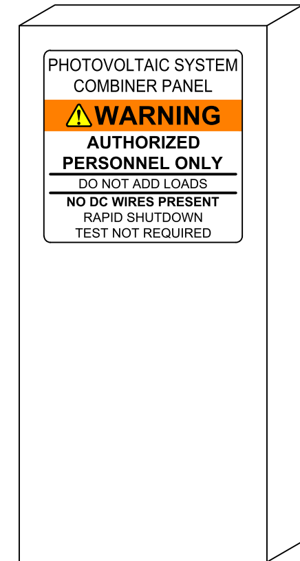
PV COMBINER BOX
