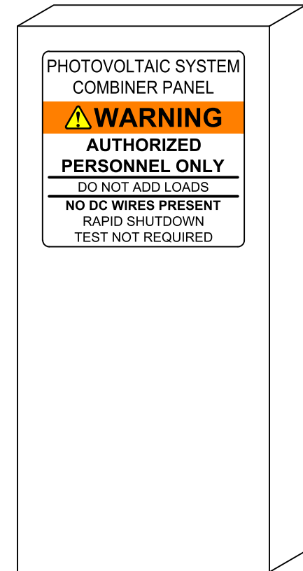
PV COMBINER BOX
