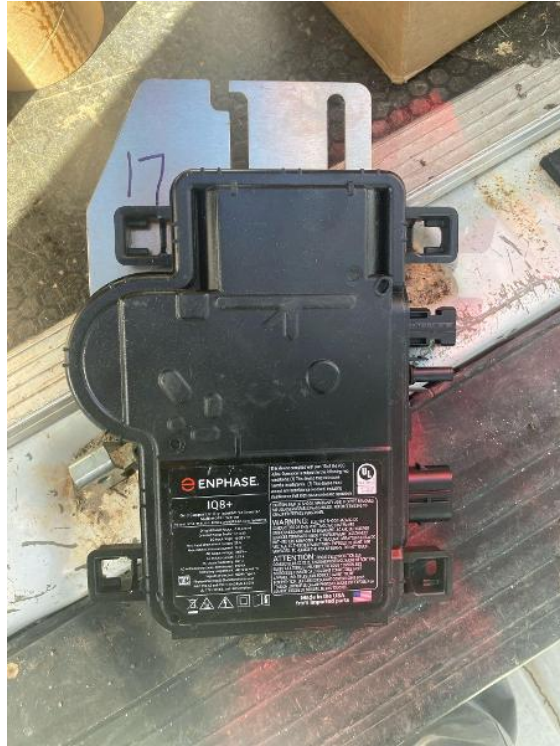
Rooftop Installation / Optimizer/ Micro Inverter Model Number
