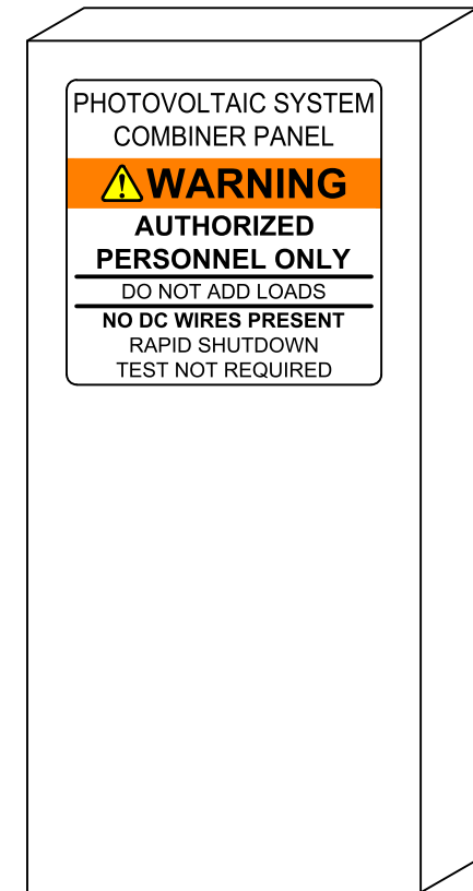
PV COMBINER BOX
