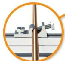
Grounding Lug A single Grounding Lug connects an entire row of PV modules to the grounding conductor.
