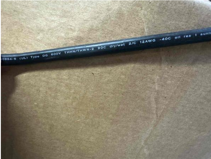
Array / Photos of Label on Trunk Cable/PV Wire
