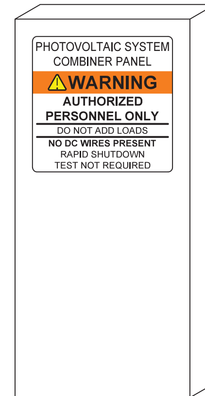
PV COMBINER BOX
