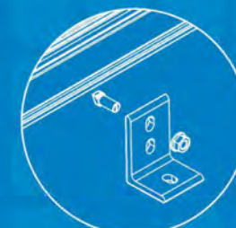
INTEGRATED BONDING MICROINVERTER MOUNT w/ WIRE MANAGEMENT
