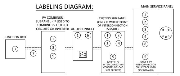
ELECTRICAL DIAGRAM SHOWN ABOVE IS FOR LABELING PURPOSES ONLY. NOT AN ACTUAL REPRESENATION OF EQUIPMENT AND CONNECTIONS TO BE INSTALLED. LABEL LOCATIONS PRESENTED MAY VERY DEPENDING ON TYPE OF INTERCONNECTION METHOD AND LOCATION PRESENTED ELECTRICAL DIAGRAM PAGE. \*\*
