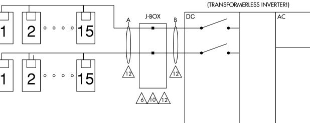
SOLAREDGE SE10000H-US W/ INTEGRATED DC DISCONNECT & INTERNAL GFDI 500VDC/240VAC, 60HZ, UL1741 W/ INTEGRATED RAPID SHUTDOWN
