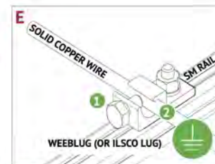
RACK SYSTEM GROUND
