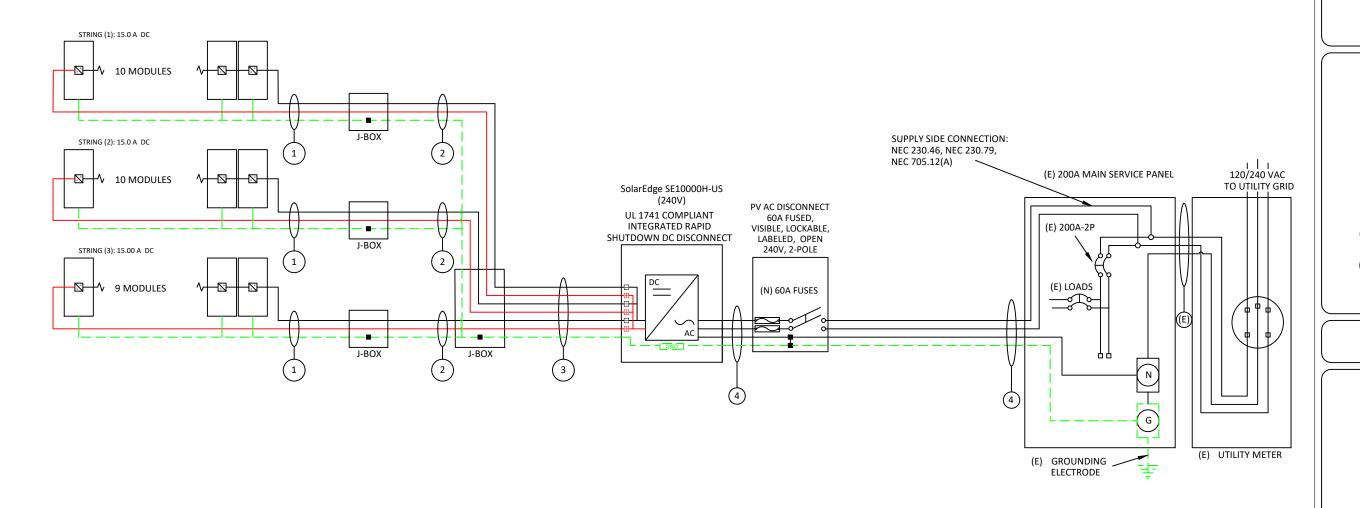
VISIBLE, LOCKABLE, LABELED AC DISCONNECT LOCATED WITHIN 10' OF UTILITY METER DRAWN BY: SoloCAD
