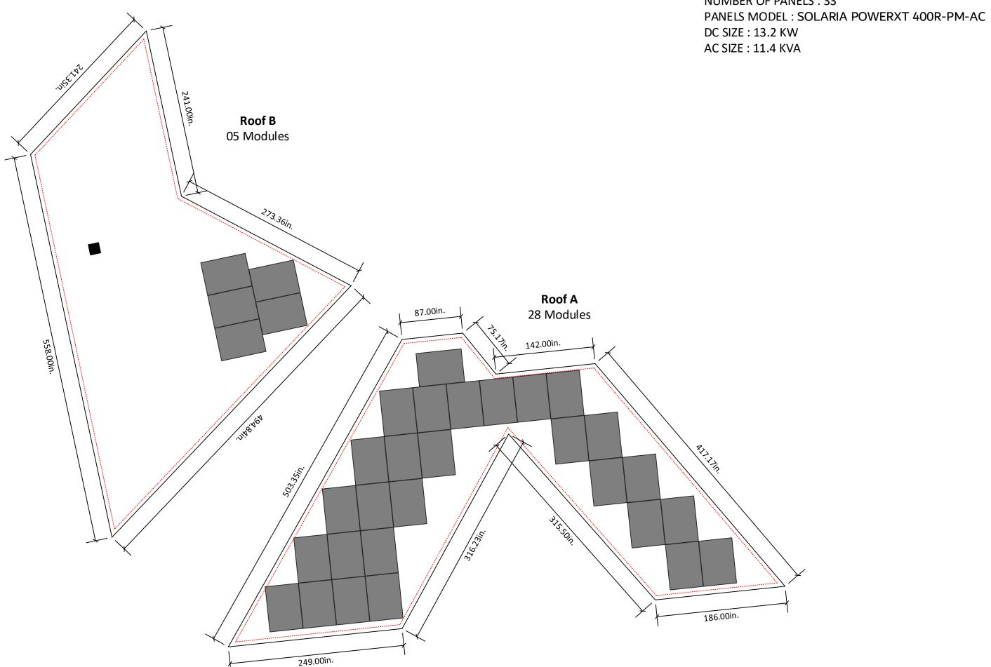
6" clearance from each side of the roof
