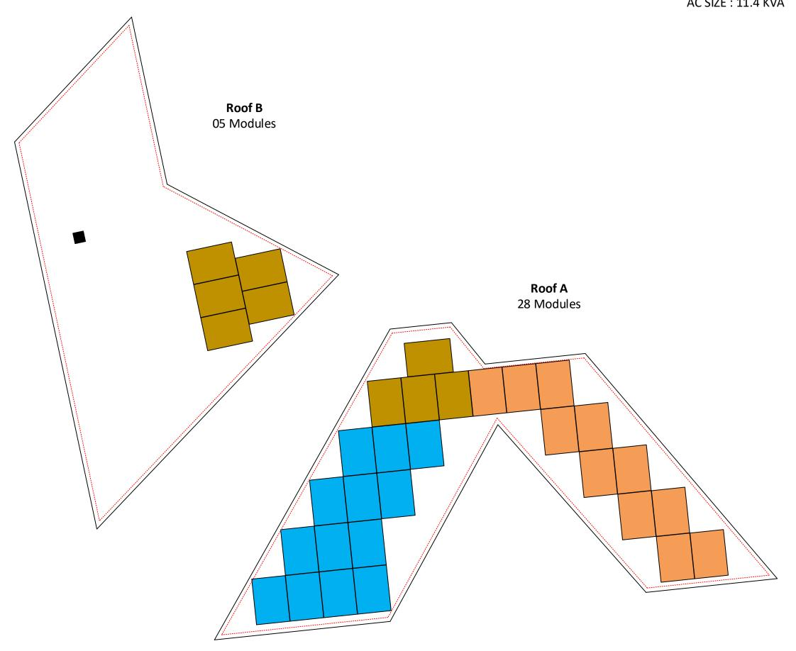
6" clearance from each side of the roof
