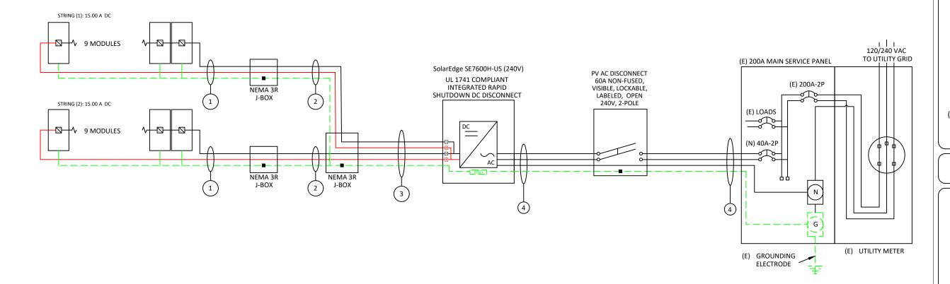
VISIBLE, LOCKABLE, LABELED AC DISCONNECT LOCATED WITHIN 10' OF UTILITY METER
