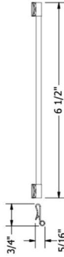
N-S BONDING PATH: N-S module to module bonding is accomplished with bonding clamp with 2 integral bonding pins. (refer also to alternate method)
