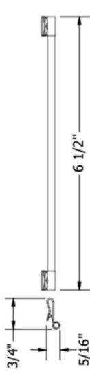
N-S Bonding Path: N-S module to module bonding is accomplished with bonding clamp with 2 integral bonding pins. (refer also to alternate method)
