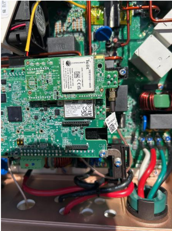
Electrical / Electrico / Inverter with Cell Kit (upper section of inverter without cover)
