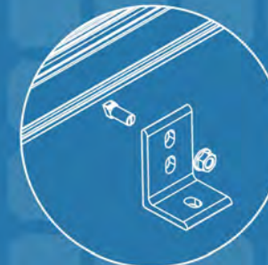
INTEGRATED BONDING MICROINVERTER MOUNT w/ WIRE MANAGEMENT
