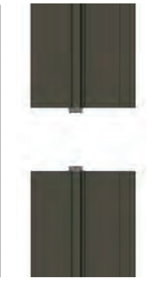
EXPANSION JOINT USED AS THERMAL BREAK W/O ELECTRICAL BONDING CONNECTION
