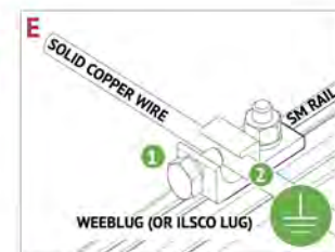
RACK SYSTEM GROUND
