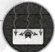
Water-Shedding Design An elevated platform diverts water away from the water seal.
