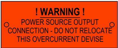
LABEL 14 AT POINT OF INTERCONNECTION OVERCURRENT DEVICE [NEC 705.12(B)(2)(3)(B)]
