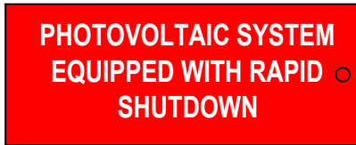
LABEL 11 AT RAPID SHUTDOWN SWITCH [NEC 690.56(C)]. LETTERS AT LEAST 3/8 INCH; WHITE ON RED BACKGROUND; REFLECTIVE [IFC 605.11.1.1]
