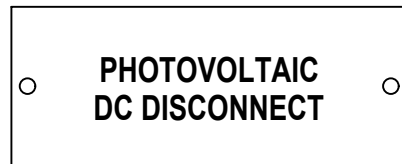
LABEL 10 AT EACH DC DISCONNECTING MEANS [NEC 690.13(B)]
