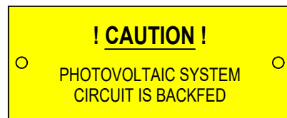
LABEL 7 AT POINT OF INTERCONNECTION; LABEL, SUCH AS LABEL 7 OR LABEL 8 MUST IDENTIFY PHOTOVOLTAIC SYSTEM [NEC 705.12(B)(4)]
