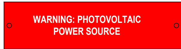
LABEL 12 AT EXPOSED RACEWAYS, CABLE TRAYS, AND OTHER WIRING METHODS; SPACED AT MAXIMUM 10 FT SECTION OR WHERE SEPARATED BY ENCLOSURES, WALLS, PARTITIONS, CEILINGS, OR FLOORS. [NEC 690.31(G)] LETTERS AT LEAST 3/8 INCH; WHITE ON RED BACKGROUND; REFLECTIVE [IFC 605.11.1.1]
