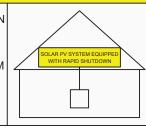
NEC 690.56 (C)(1)(a) PLACE WITHIN 3FT OF SERVICE DISCONNECTING MEANS TO WHICH THE PV SYSTEMS ARE CONNECTED AND SHALL
