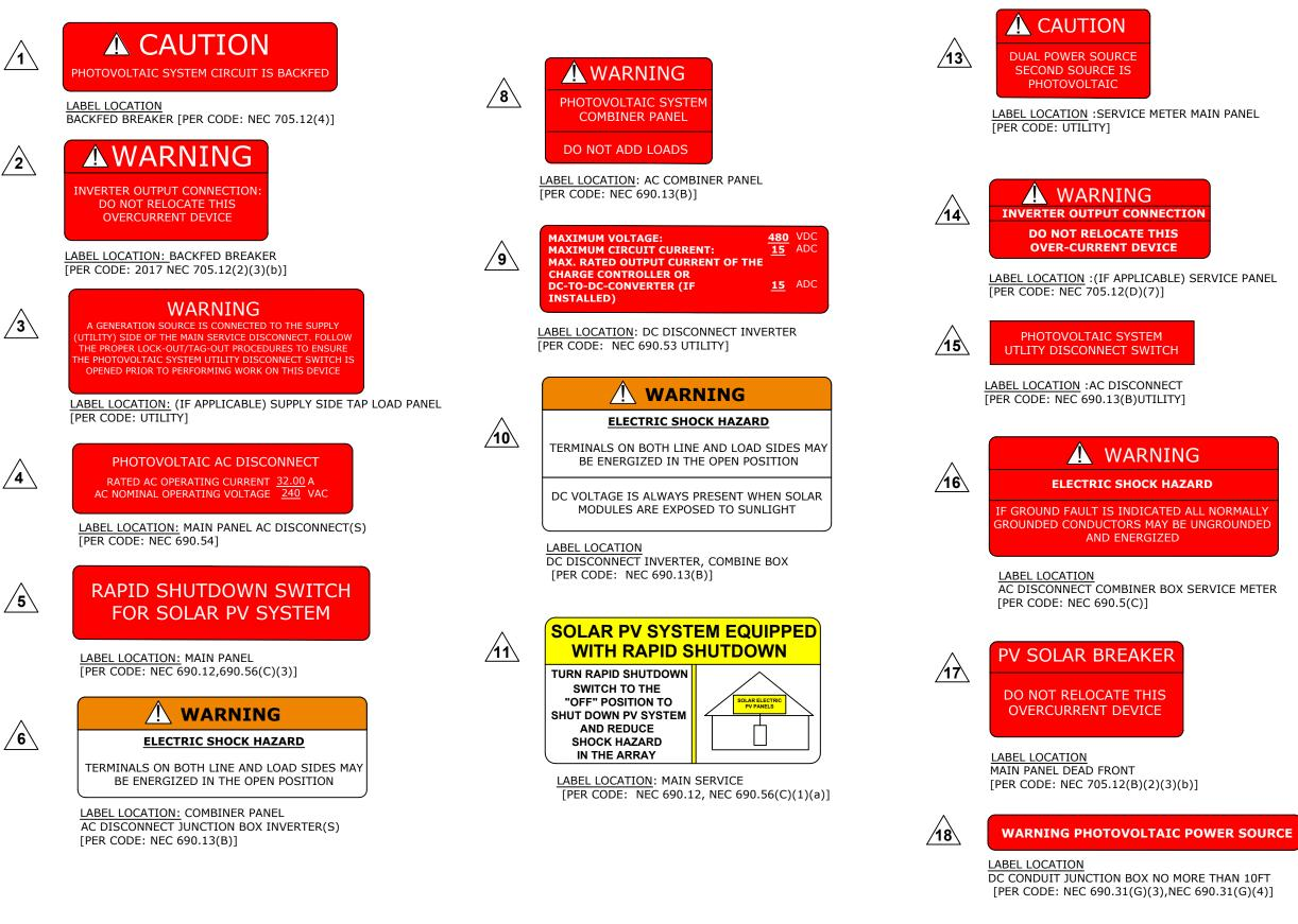
REFLECTIVE AND WEATHER RESISTANCE LABEL REQUIRES CAPITALIZED LETTERS WITH A MINIMUM HEIGHT OF 3/8INCH, WHITE LETTERS ON RED BACKGROUND LABELS SHALL BE PLACED ON INTERIOR AND EXTERIOR DCCONDUIT, RACEWAYS, ENCLOSURE, AND CABLE ASSEMBLIES EVERY 10 FEET, WITHIN 1 FOOT OF TURNS OR BENDSAND WITHIN 1 FOOT ABOVE AND BELOW PENETRATIONS OF ROOF/ CEILING ASSEMBLIES, WALLS OR BARRIERS.
