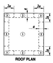
Roof Zones for Buildings with h > 60 ft. (for Gable Roofs <=  $10^{\circ}$  and Monoslope Roofs <=  $3^{\circ}$ )
