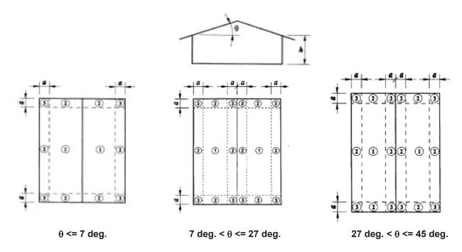
Roof Zones for Buildings with h <= 60 ft. (for Gable Roofs <= 45° and Monoslope Roofs <= 3°)
