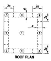
Roof Zones for Buildings with h > 60 ft. (for Gable Roofs <=  $10^{\circ}$  and Monoslope Roofs <=  $3^{\circ}$ )
