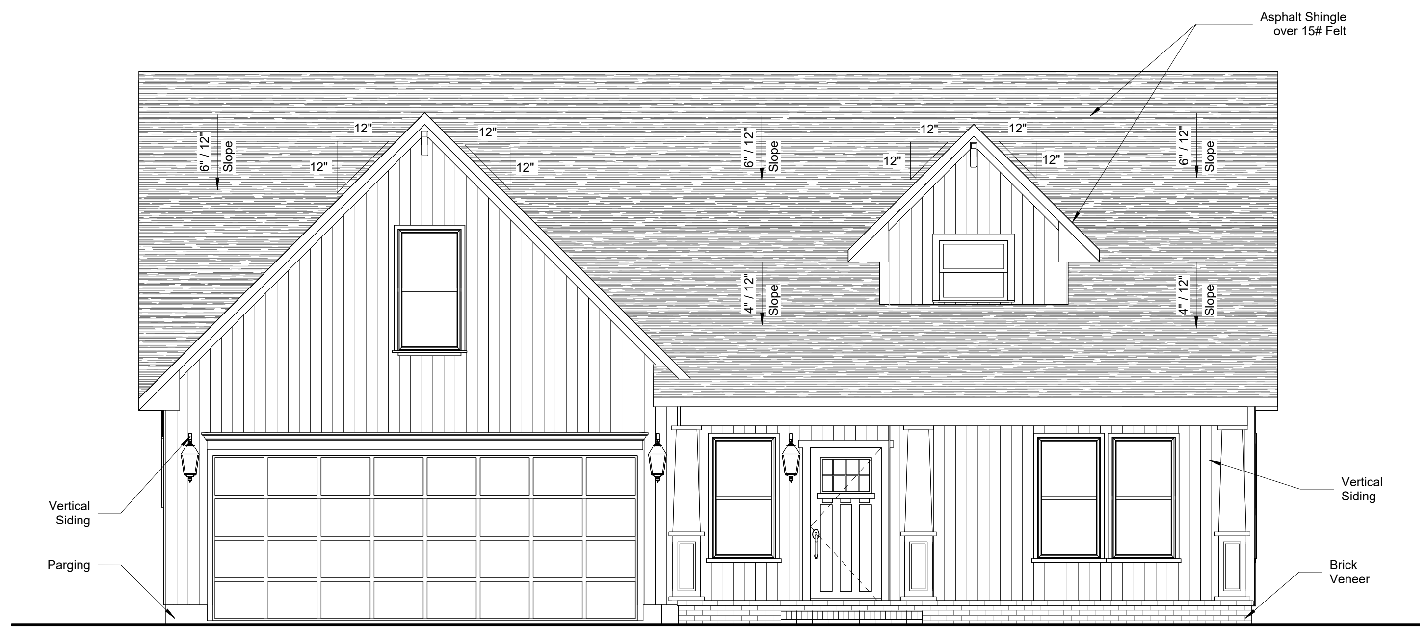
① Front Elevation 1/4" = 1'-0"
