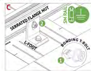
RAIL TO L-FOOT w/BONDING T-BOLT
