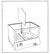
Separate the two sections by sliding the partition piece into the left slots.
