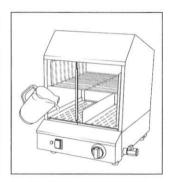
Pour 8 quarts of hot water into the unit's base, covering the heating elements.
