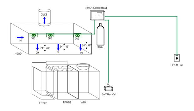
System is a Pyrochem PCL 300 wet chemical system with a 10 flow point capacity. This application uses 7 flows. Hood and system are existing. Tank size is being changed to accommodate new equipment.
