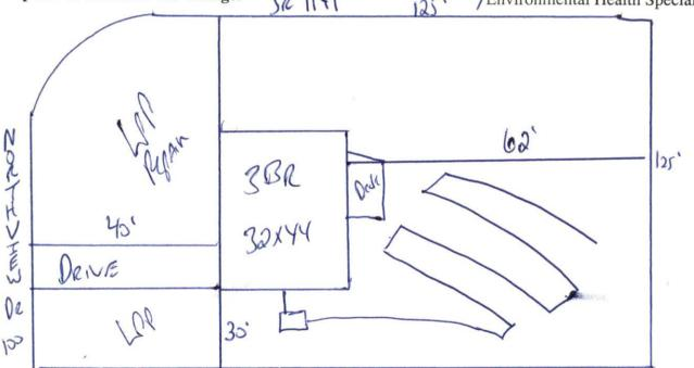
STUB Out Plumbing shallow where shown - 18 dy Ditch Dophis MAINTAIN All set Backs Do not drive or pack on systemsystem
