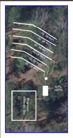
System: Gravity to D-Box Lines: 1-3 (210')
