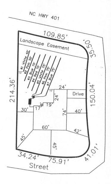
System: Gravity to D-Box Lines: 5-7 (225') 0.4 LTAR 24" Trench Bottom Accepted Status System Repair: serial distribution Lines: 1-4, (230') 0.4LTAR 24" Trench Bottom Accepted Status System
