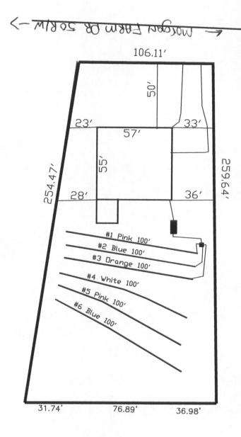
System: Gravity to D-Box Lines: 1-3, (300') 0.4 LTAR 24" Trench Bottom Accepted Status System Repair: Gravity to D-Box Lines: 4-6, (300') 0.4LTAR 18" Trench Bottom Accepted Status System
